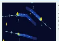
Clearly identifies moving targets from Showing past position with 5 dots for stationary targets. The display shows the TT targets and AIS targets. exact movement of other vessels like drawing tails. Even when your range PAST POSN TIME is changed, a new trail appears past drawing tails. 3 types of shape are available.
