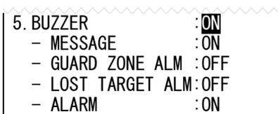
Setting of Buzzer functions
